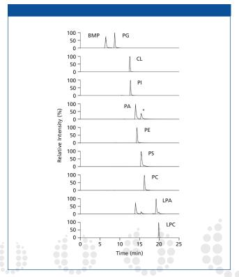
**Figure 2:** Separation of PL standards in ascending retention order with iHILIC®-Fusion. \*Double peak of PA is caused by in-source fragmentation of the PS head group resulting in corresponding PA species.
