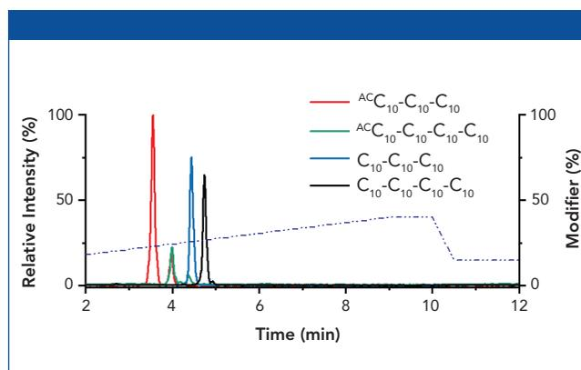
**Figure 2:** SFC MS chromatogram of four different exophilins detected as sodium adduct ( $[M+Na]^+$ ): C<sub>10</sub>-C<sub>10</sub>-C<sub>10</sub>-C<sub>10</sub>  $m/z$  599.4, <sup>Ac</sup>C<sub>10</sub>-C<sub>10</sub>-C<sub>10</sub>-C<sub>10</sub>  $m/z$  641.4, C<sub>10</sub>-C<sub>10</sub>-C<sub>10</sub>-C<sub>10</sub>  $m/z$  785.5, <sup>Ac</sup>C<sub>10</sub>-C<sub>10</sub>-C<sub>10</sub>-C<sub>10</sub>  $m/z$  827.5.
